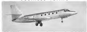
ENGINE INLET location on Jetstar gives good run recovery at all attack angles because wing sets in flow straightening zone.
